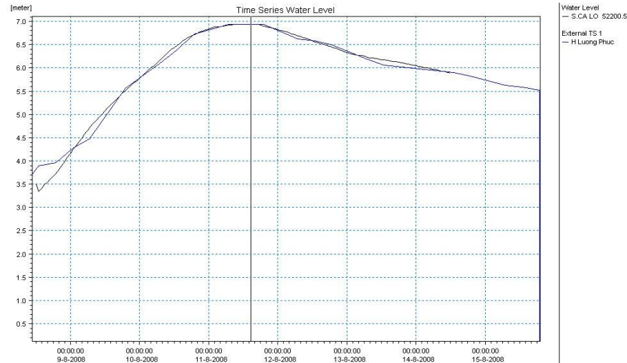
Figure 5: Results of model testing at Phuc Luong According to measured data from 9 to August 14, 2008
